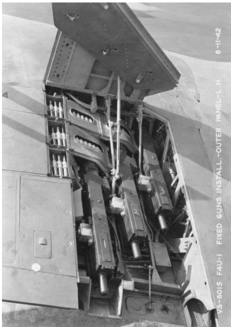
Three Browning .50-caliber machine guns and belted ammunition installed in the left wing of a Vought-Sikorsky F4U-1 Corsair, 11 August 1942. (Vought-Sikorsky)
