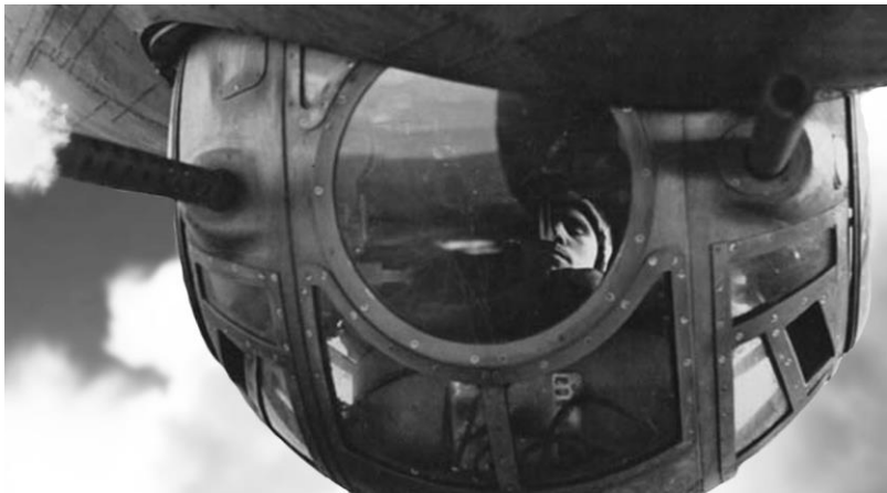
A gunner fires the two Browning .50-caliber machine guns of a B-17's ball turret. (U.S. Air Force)
