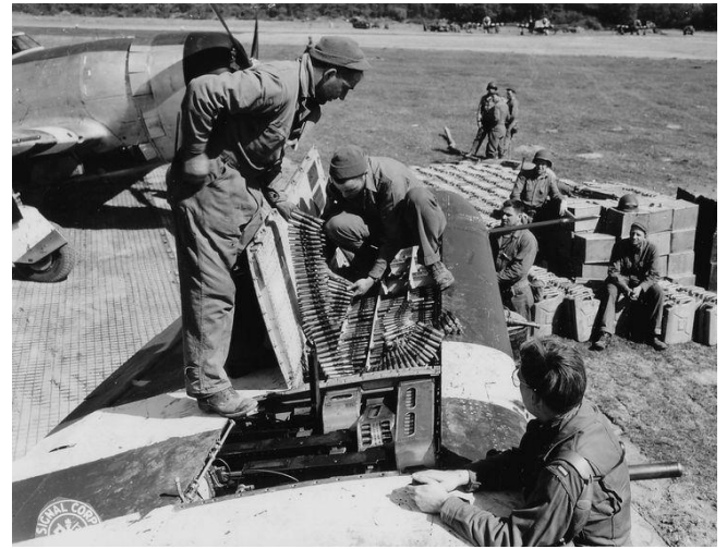
Armorers load disintegrating-link belts of .50-caliber ammunition for the eight machine guns of a Republic P-47 Thunderbolt. (U.S. Air Force)
