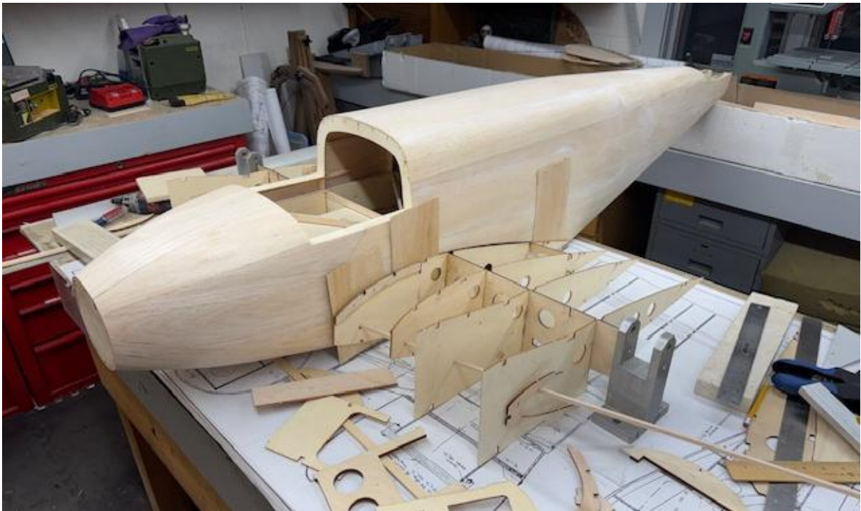
Len Buffintin is currently building a Zirolli Beechcraft 18. See page 16-19 for details and pictures.
