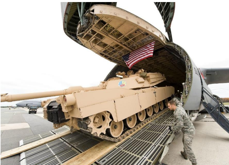
An M1A1 Abrams Main Battle Tank being loaded on the forward cargo ramp of a Lockheed C-5M Super Galaxy. The transport's nose has been raised to provide loading access from the front of the airplane. The tank weighs 139,081 pounds (63,086 kilograms). (Roland Balik/U.S. Air Force)
